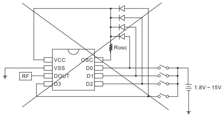
Warning: Be cautious to use this circuit which will cause the IC shutdown or even damaged.
