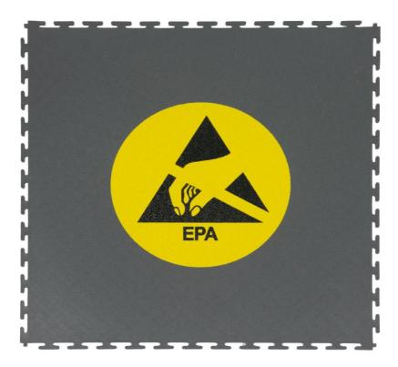
These interlocking floor tiles are made of PVC and during the molding process metal particles are injected. That way a very homogenic and durable conductive effect is generated, lasting the full lifetime of the product, considering wear and tear, unless correctly maintained by cleaning with antistatic floor cleaner.
