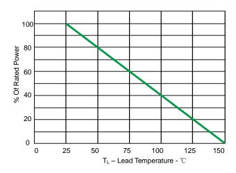
Fig 2.Power Derating Curve
