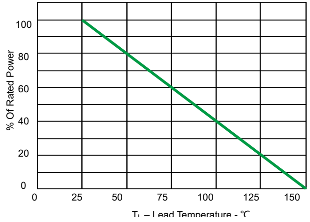
Fig 2. Power Derating Curve
