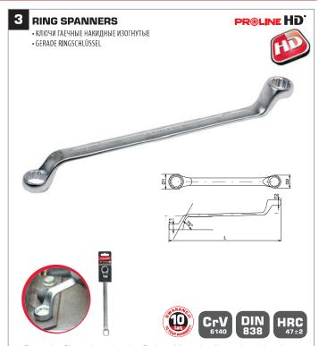
• Forged • Chromium-plated • Satin • Meet the dimension-related requirements of German DIN 3110 standard • The maximum torque is 60% higher than in German DIN 899 and in US ANSI standard
