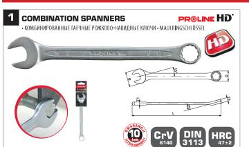
• Forged • Chromium-plated • Satin • Meet the dimension-related requirements of German DIN 3113 standard ullet The maximum torque is 60% higher than in German DIN 899 and in US ANSI standard
