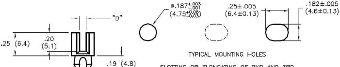
SLOTTING OR ELONGATING OF 2ND AND 3RD MOUNTING HOLE IS RECOMMENDED TO ALLOW FOR LENGTH VARIATIONS IN MOLDING AND ASSEMBLY EASE.
