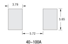
20A-30A: Recommend trace thickness is 3oz, the minimum trace width is 10mm 40A-50A: Recommend trace thickness is 3oz, the minimum trace width is 15mm 60A-70A: Recommend trace thickness is 3oz, the minimum trace width is 22mm 80A-100A: Recommend trace thickness is 6oz, the minimum trace width is 33mm
