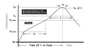
**Wave Soldering:** 260°C, 10 seconds max. **Infrared Reflow:** 260°C, 30 seconds max.
