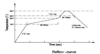
Recommended reflow methods:IR,hot air oven ,nitrogen oven Devices can be cleaned using standard industry methods and solvents. **NOTE:**
