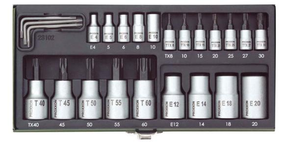
This set contains 1/4" drive (6.3mm) TX sockets in sizes TX8 to TX30 (with frontal hole) and external TX sizes E4 to E8 (all suitable for tightening torques up to 25Nm), 1/2" drive (12.5mm) TX sockets in sizes TX40 - 60 and external TX E10 to E18 (for tightening torques from 25 to 135Nm) and three offset TX spanners - the TX6, 8 and 10. See photo for full contents.
