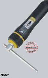
A well-shaped ergonomic screwdriver handle allows for torques from 6 to 8Nm just by manual operation. For higher torques, the MC 10 has a 1/4" square connector on the rear end for fitting a lever (T-handle, ratchet).
