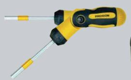
Locking of the handle in normal and angled position at the push of a button. Reverse lever for clockwise and anticlockwise rotation by turning the shift ring. In centre position the ratchet function is eliminated. Autolock system: Bits are form-locked automatically when inserted by means of a spring and a magnet. To release, slide ejector backwards.
