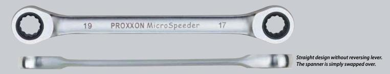
Often used for demounting engines, working on automatic transmissions, rear axles, etc. Ratcheting function with 72-teeth inner gear ring, made of high alloy special steel allowing ratcheting even when the spanner can only be moved through 5°. Shaft of CrV steel with optimum surface protection: double nickel-plating and single matt-finished chrome-plating. With durable laser marking and easy-to-read sizes.
