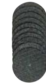
NO 28 808 10 pieces Aluminium oxide cutting discs with reinforcement The cutting discs are available in Ø 22 x 0.8 and Ø 38 x 1. Nearly unbreakable, making them usable to remove stock. Will cut alloyed, standard and stainless steels, non-ferrous metals and even wood and plastic. Arbor shaft of Ø 2.35.
