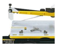
**Patented saw blade holders with high clamping force** ensure true alignment of the saw blades. Recesses in the table surface serve as guide line in assembly to define position and distance of the saw blade holders.
