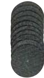
NO 28 808 10 pieces Aluminium oxide cutting discs with reinforcement The cutting discs are available in Ø 22 x 0.8 and Ø 38 x 1. Nearly unbreakable, making them usable to remove stock. Will cut alloyed, standard and stainless steels, non-ferrous metals and even wood and plastic. Arbor shaft of Ø 2.35.
