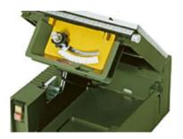
Table and drive can be lifted up and supported like an engine bonnet. For cleaning the device and easy saw blade replacement.
