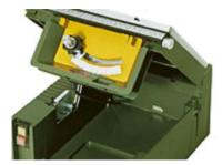
Table and drive can be lifted up and supported like an engine bonnet. For cleaning the device and easy saw blade replacement.
