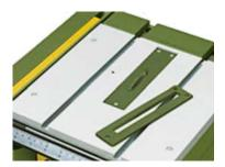
Non-slotted sawing cap cover of ABS for tight tolerances between saw blade and table (is slotted from below by the FET saw blade). For cutting very small parts.
