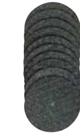
NO 28 808 10 pieces Aluminium oxide cutting discs with reinforcement The cutting discs are available in \varnothing 22 x 0.8 and \varnothing 38 x 1. Nearly unbreakable, making them usable to remove stock. Will cut alloyed, standard and stainless steels, non-ferrous metals and even wood and plastic. Arbor shaft of \varnothing 2.35.
