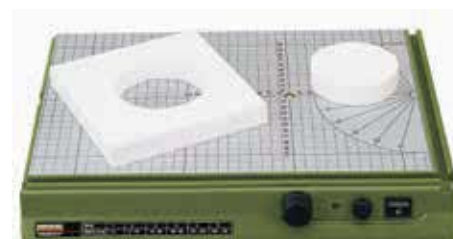
Crosscuts are achieved by means of a simple yet efficient solution: secure drawing-pin to table by means of tape, it serves as a fixed centre.
