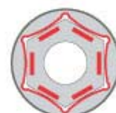
The Driver-System: The driving force is applied to the flanks, not the corners.
