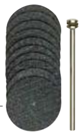
NO 28 808 10 pieces Aluminium oxide cutting discs with reinforcement The cutting discs are available in Ø 22 x 0.8 and Ø 38 x 1. Nearly unbreakable, making them usable to remove stock. Will cut alloyed, standard and stainless steels, non-ferrous metals and even wood and plastic. Arbor shaft of Ø 2.35.
