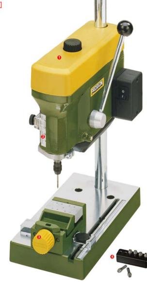
**1** 3 spindle speeds by shifting the flat belt for more than the triple torque in the lower rotational speed range.
