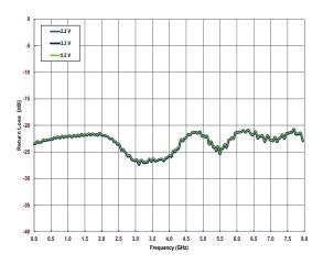
Figure 8 • Isolation vs.  $V_{DD}$  (RFC-RFX)
