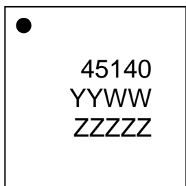
Figure 19. Top Marking Specifications
