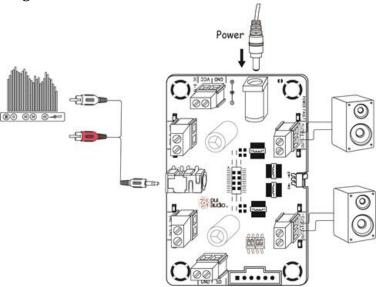
The gain on this amplifier board is fixed at 26 dB. Please use your audio source device's volume control to adjust the amplifier output. Alternatively, you can connect a 25 kOhm audio taper potentiometer between the audio source device and amplifier for the purpose of volume control.
