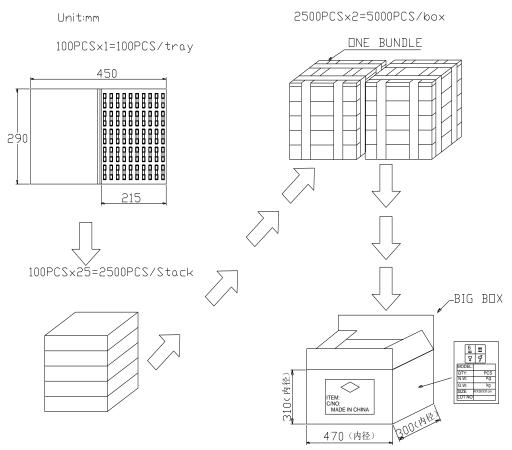
Unless otherwise specified, tolerance: ±10(unit:mm)
