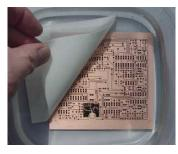
The circuit image is laid face-down over the copper-clad surface and subjected to high heat and pressure (using either a calibrated houshold iron or the highly recommended "laminator" (see right-panel >) upon which, the toner image will re-fuse to the copper's surface. The board and paper combination are then submerged in a tray of water where
