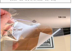
Shown with Carrier Board supporting printed page ovelaid with foil, passing through the laminator.
