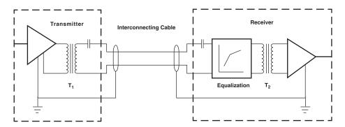
T<sub>1</sub>, T<sub>2</sub>: PE-65612 or PE-65812
