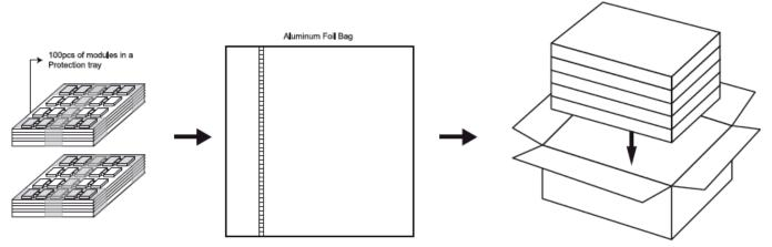
Pack 2 Protection trays (200pcs of modules) into an Aluminum Foil Bag. Seal the Aluminum Foil Bag. 2. Pack 5 Aluminum Foil Bags with the modules into a carton box (1000pcs in total).
