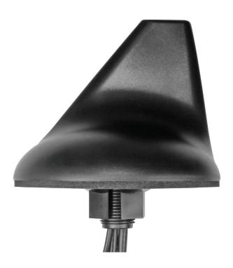
Pulse is proud to introduce a new state-of-the-art direct mount multi band antenna. This body mount antenna operates from 698 thru 2700 MHz, including LTE. The antenna is ideal for voice, mobile data, Public Safety, WLAN and asset tracking applications. The rugged, yet aesthetically pleasing design provides UV and IP-65 protection to ensure a long, reliable, maintenance-free life.
