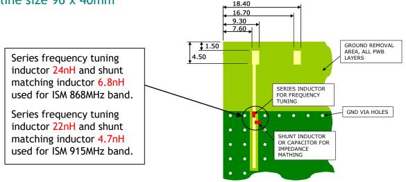
Feed line should be designed to match 50  $\Omega$  characteristic impedance, depending on PWB material and thickness.
