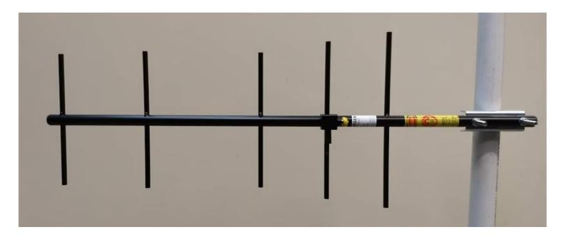
Antenna mounted vertically on post with gamma rod facing down
