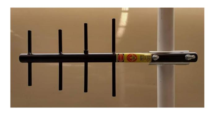
Antenna mounted vertically on post with insulator on driven element facing up
