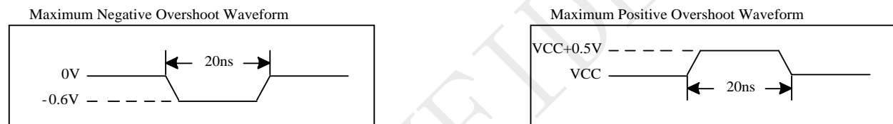
Figure 5-1 Maximum Overshoot Waveform
