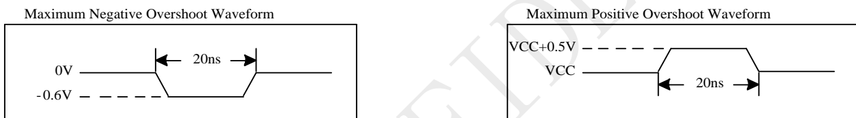
Figure 5-1 Maximum Overshoot Waveform
