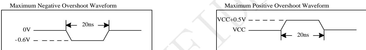
Figure 5-1 Maximum Overshoot Waveform
