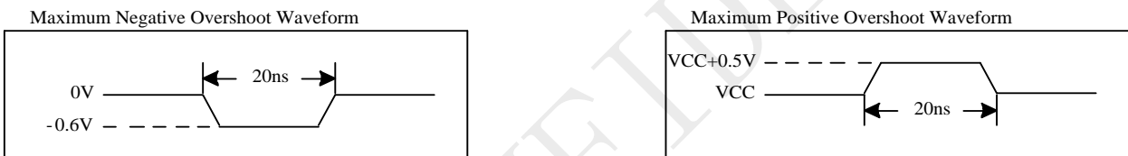
Figure 5-1 Maximum Overshoot Waveform
