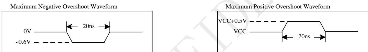
Figure 5-1 Maximum Overshoot Waveform
