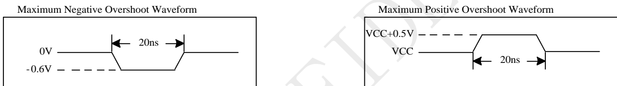
Figure 5-1 Maximum Overshoot Waveform
