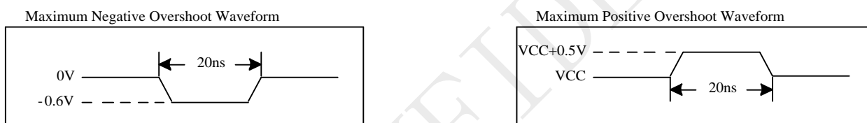
Figure 5-1 Maximum Overshoot Waveform
