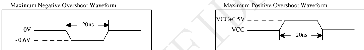
Figure 5-1 Maximum Overshoot Waveform
