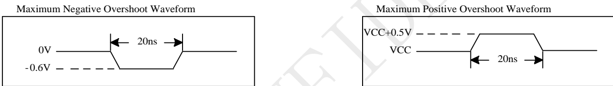
Figure 5-1 Maximum Overshoot Waveform
