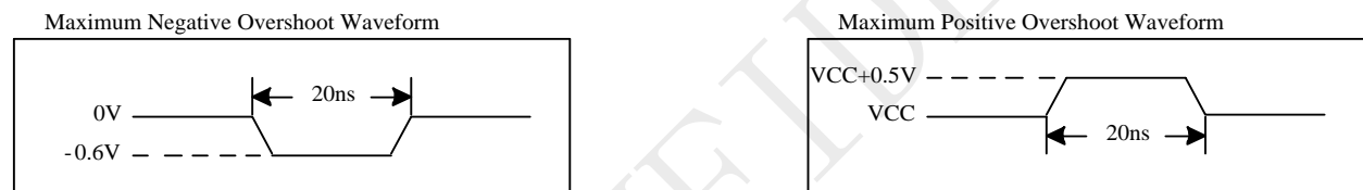
Figure 5-1 Maximum Overshoot Waveform
