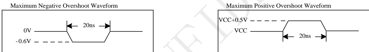
Figure 5-1 Maximum Overshoot Waveform
