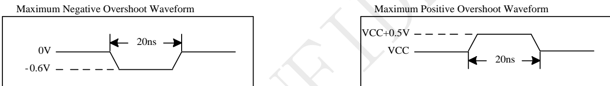
Figure 5-1 Maximum Overshoot Waveform
