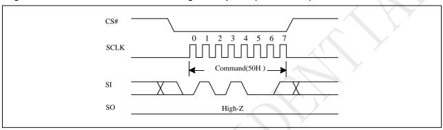
Figure 10-4 Write Enable for Volatile Status Register Sequence (Command 50)
