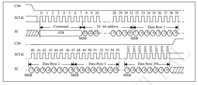
Figure 10-26 Program Security Registers (PRSCUR) Sequence (Command 42)
