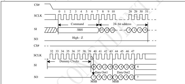
Figure 10-10 Dual Read Mode Sequence (Command 3B)
