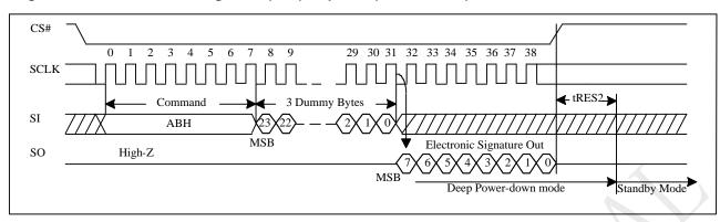
Figure 10-29 Read Electronic Signature (RES) Sequence (Command AB)
