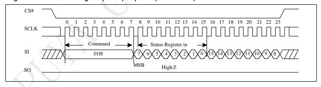
Figure 10-7 Write Status Register (WRSR) Sequence (Command 01)
