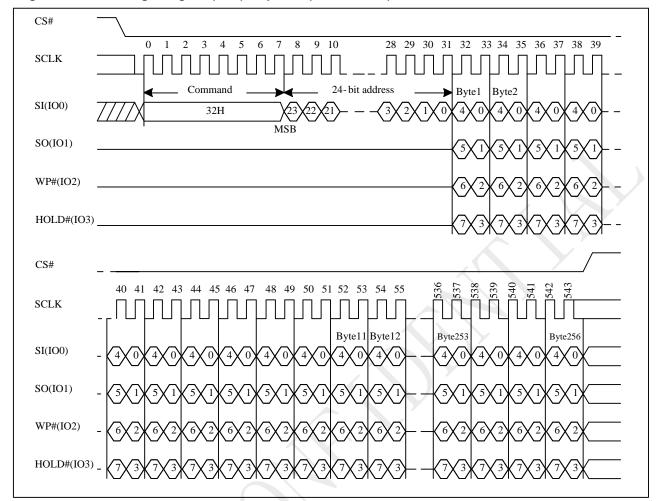
Figure 10-24 Quad Page Program (QPP) Sequence (Command 32)
