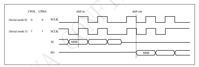
Figure 8-1 Serial Peripheral Interface Modes Supported
