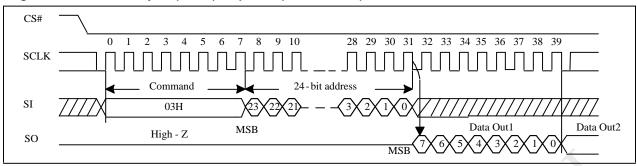
Figure 10-8 Read Data Bytes (READ) Sequence (Command 03)
