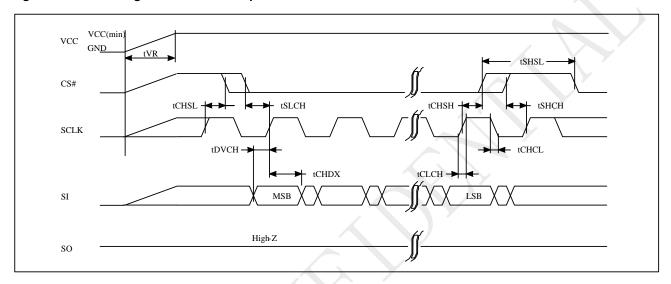
Figure 5-9 Power-up Timing
