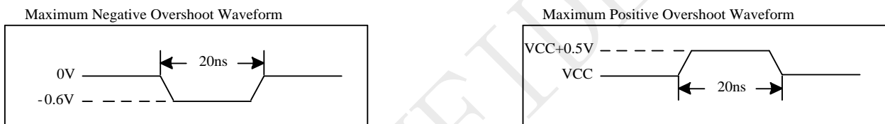
Figure 5-1 Maximum Overshoot Waveform
