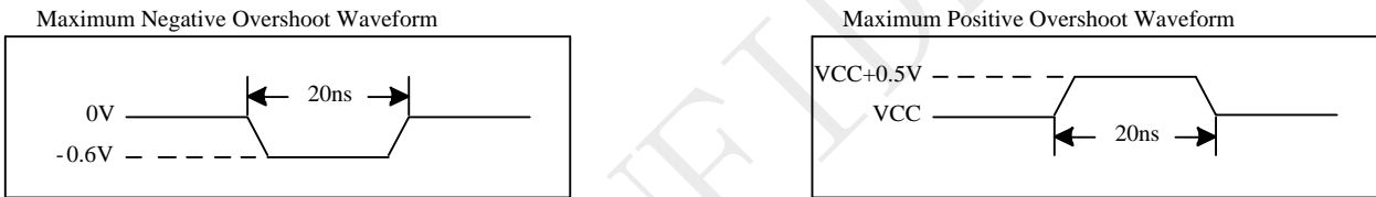
Figure 5-1 Maximum Overshoot Waveform
