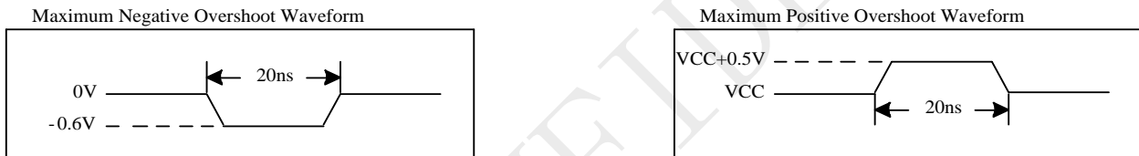
Figure 5-1 Maximum Overshoot Waveform
