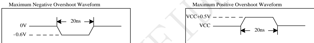
Figure 5-1 Maximum Overshoot Waveform
