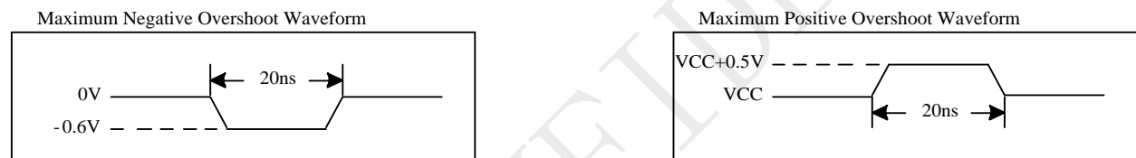
Figure 5-1 Maximum Overshoot Waveform
